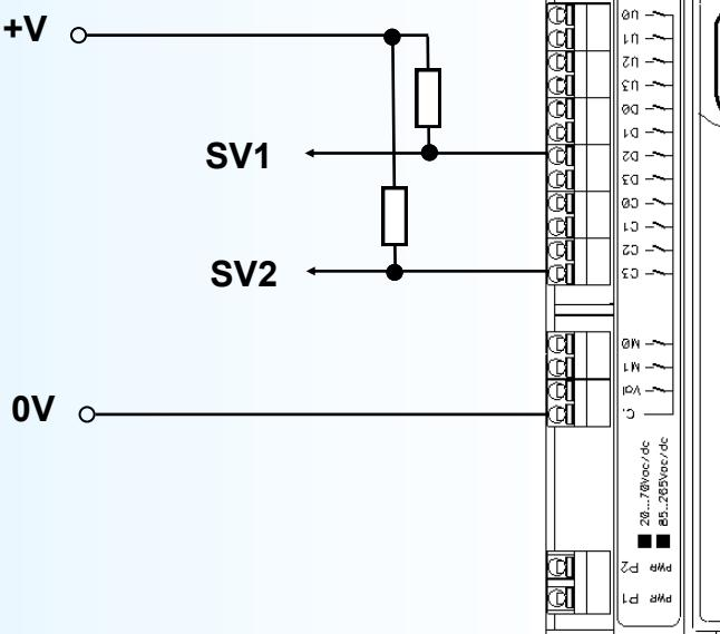
Notes: The resistors are used for limit the current through the static relays outputs.
