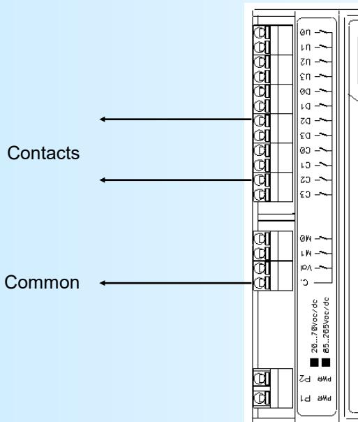
In <NORMAL> logic, The outputs contacts are "open" and "close" when the outputs are active.
